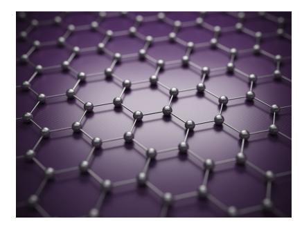
Graphene is a unique carbon structure. It consists of a single atom layer of carbon atoms arranged in a honeycomb lattice and is the world's first two-dimensional (2D) material. Graphene boasts exceptional properties, highly valuable to the semiconductor industry, including:
