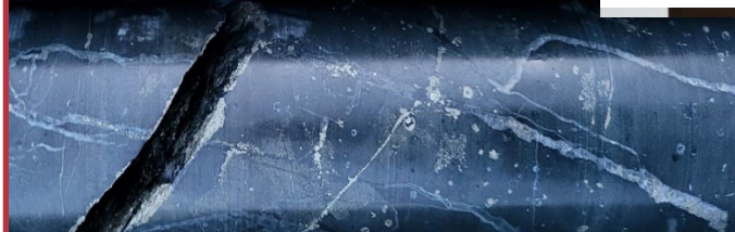
SPD003 419.8m, pyrite stringer stockwork/multiple vein sets associated with silica alteration, 1.42g/t Au (Epithermal)
