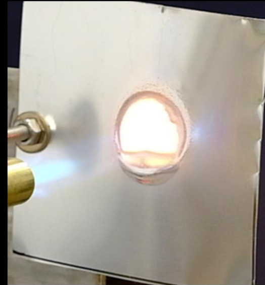
UNCOATED ALUMINIUM 15 seconds under butane flame
