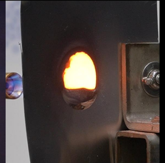
UNCOATED ALUMINIUM 15 seconds under butane flame
