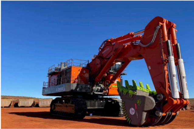
Figure 14 – Mainetec’s Hulk excavator bucket
