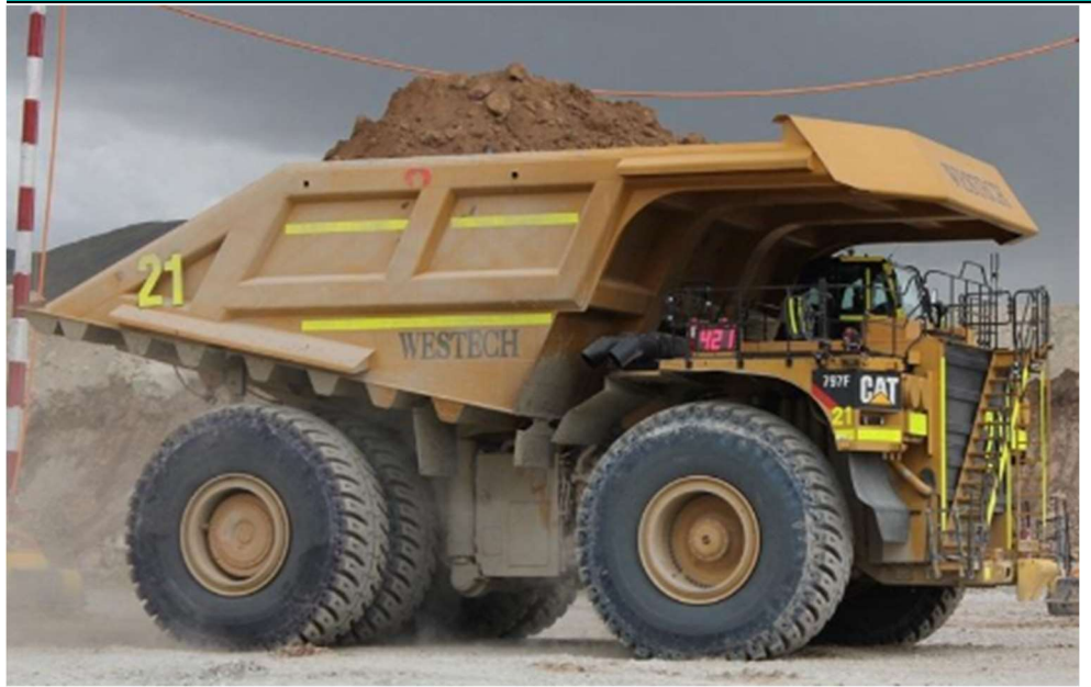
Figure 12 – A Cat 797F with an Austin Westtech truck body
