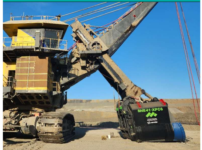
Figure 17 – Dipper Bucket mounted
