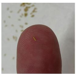
Single Cell sorting made possible by precision PEEK extrusion; 250um ID, 360um OD, concentric, 2-4mm length.
