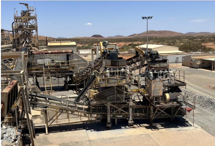
Crushing circuit: 100tph – proof run (operational)
