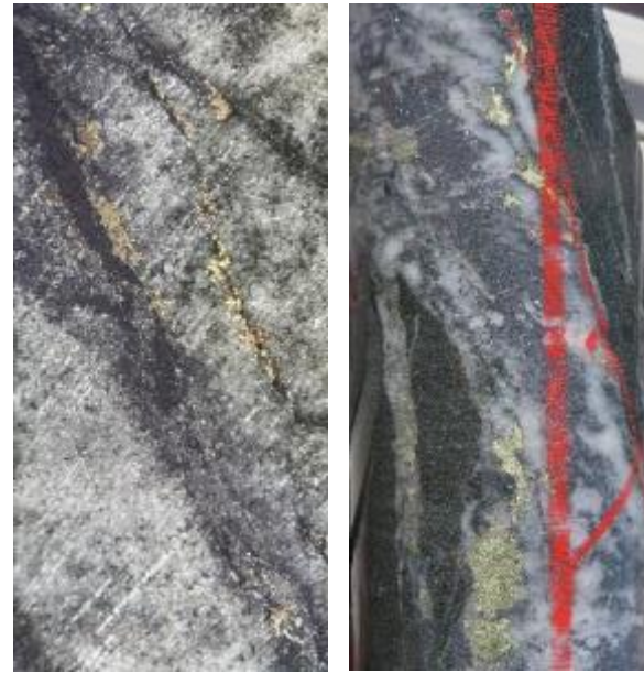
Osprey IOCG Mineralisation (Chalcopyrite, pyrite) No gold assays to date
