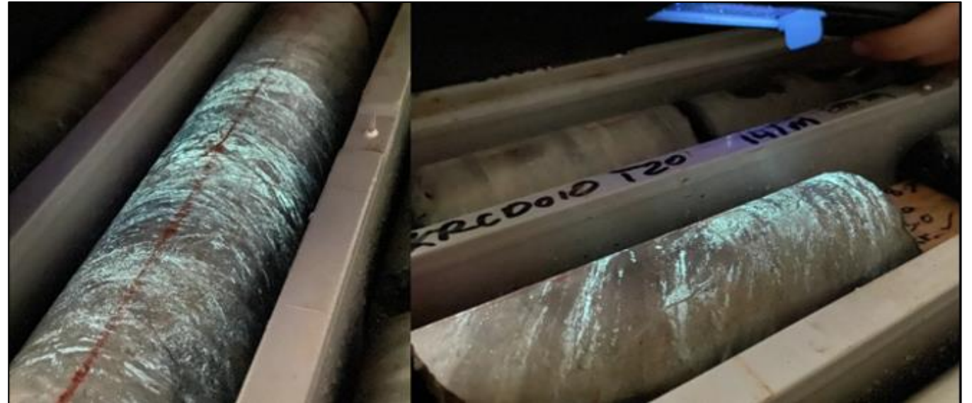
Bornite (copper sulphide) with malayaite (calcium-tin-silicate) fluorescing under UV light in 3KRC0010. Drillcore is 61.1mm wide for scale.
